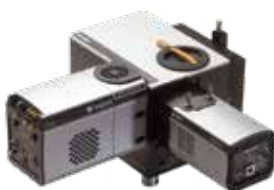
Kymera 19 193 mm focal length & F/3.6 aperture
